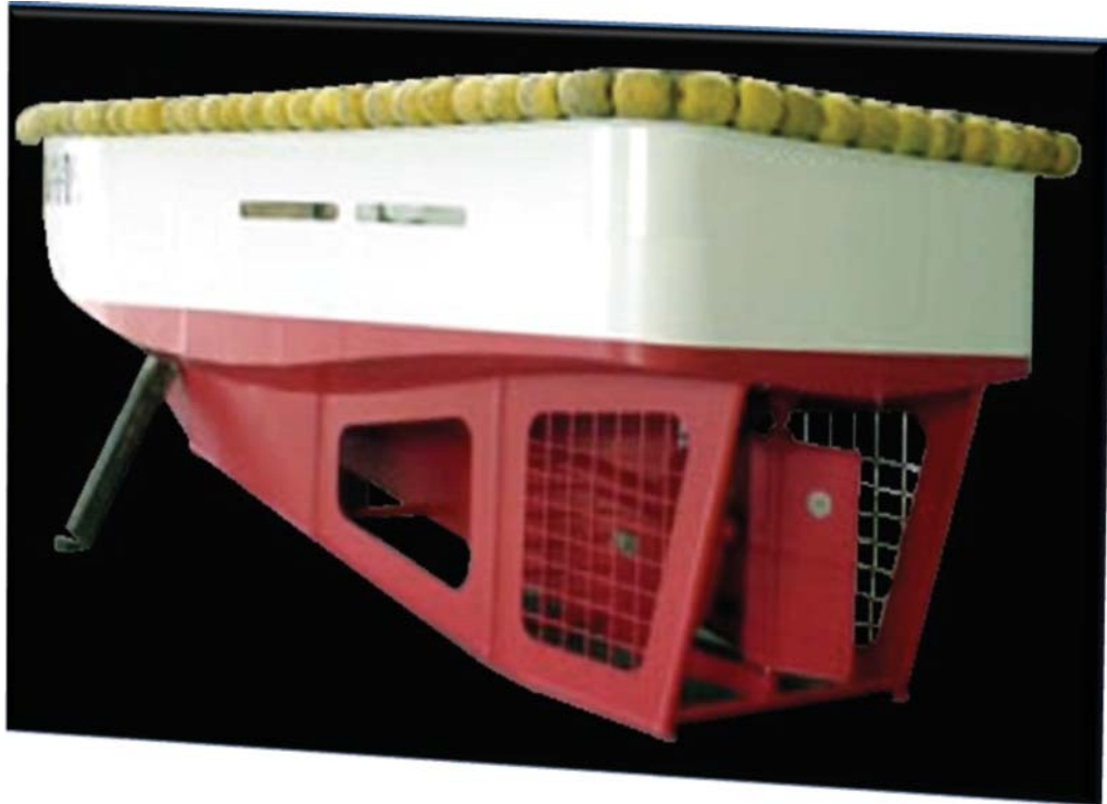
Figure 015: Spanish designed and manufactured 250hp BFT purse seining skiff used onboard by most last generation Mediterranean Sea BFT purse seine fishing vessel.
