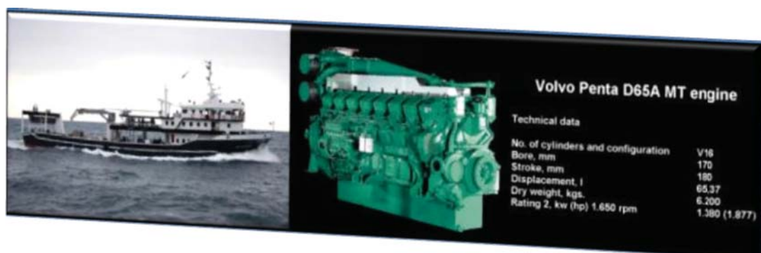
Figure 008: Turkish flagged BFT PS Vessel DENIZAR (LOA: 51m) built by Ba aran Gemi and equipped with a Volvo Penta D65A Mt engine.
